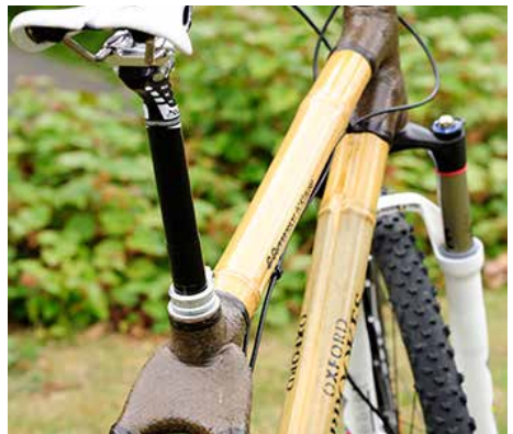
Close up of the Bamboo Bike and flax joining technology
